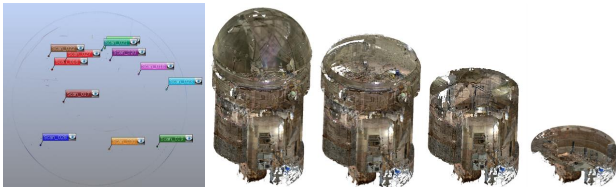
Figure 8. Point cloud of a part of the Belgian Reactor 3 (BR3), showing the different levels (BR3) [11]
