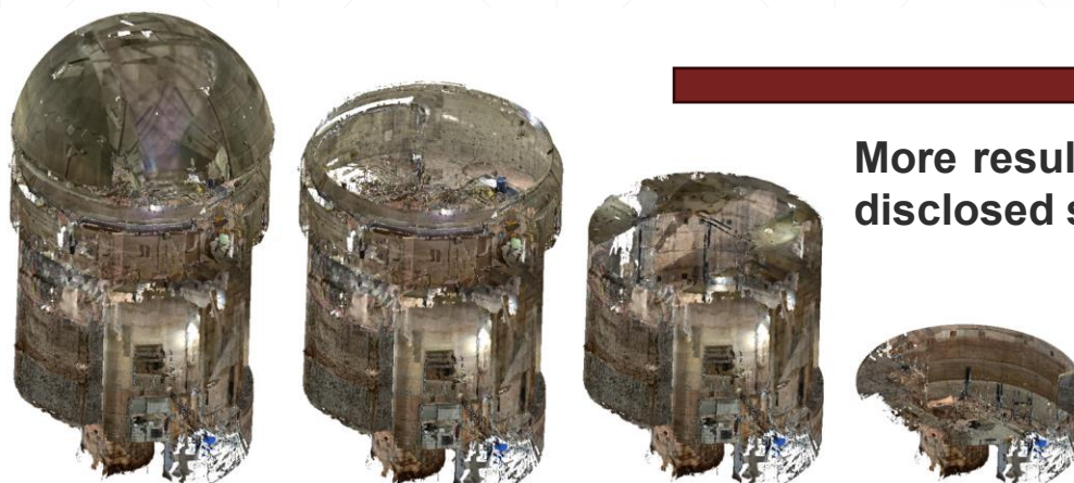
Figure 13. Processing of scans with SCENE Software (left) and point cloud of a part of the BR3, showing different levels (right) [11]
