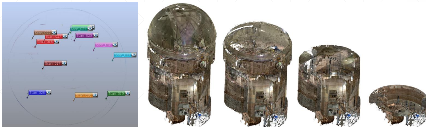
Figure 13. Processing of scans with SCENE Software (left) and point cloud of a part of the BR3, showing different levels (right) [11]
